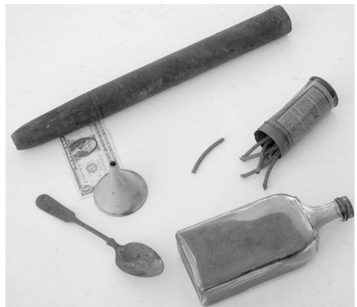
The splitting gun, fuses, funnel and spoon, and a jar of black powder with the dollar bill shown for size. Courtesy of Carlton Lewis, photo by Gerry Stoner.
